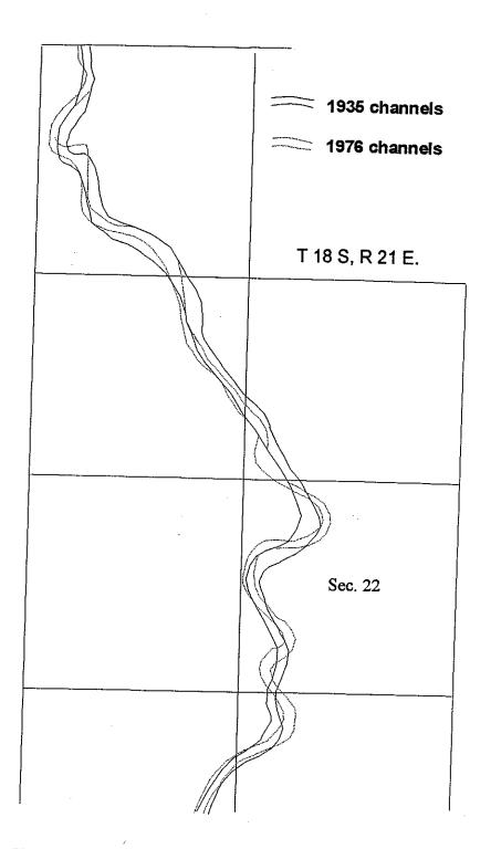
Figure 3. Channel changes in upstream from St. David, upper San Pedro River. Channel postions were documented using aerial photographs from 1935 and 1972. Channels in 1972 are shown only where they are different from those of 1935. Note the increased meander development in the southern portion of the map area. Section boundaries are shown by fine vertical and horizontal lines.
